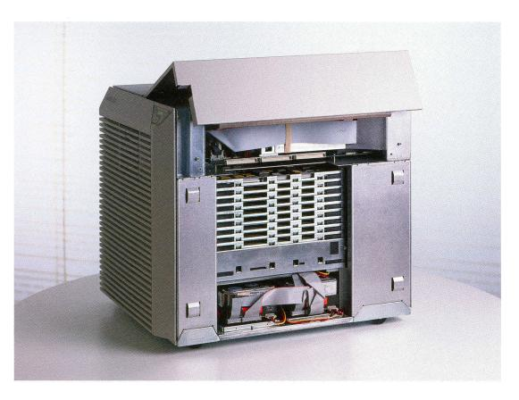
The interior of the Series 10000 reflects its highly efficient design and easy accessibility. datapaths as to the CPUs. As a result, the Series 10000 solves one of the key problems in multiprocessor systems: the capacity of the memory bandwidth to handle massive information flow. That's why Apollo engineers made sure the Series 10000 could easily meet the demands of today's high-throughput applications.
