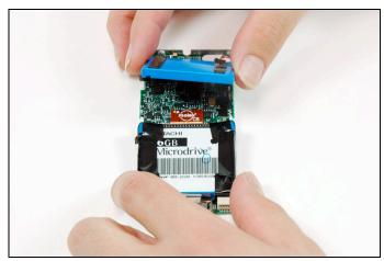
Lift the battery off of the logic board and lay it to the side of the iPod.
