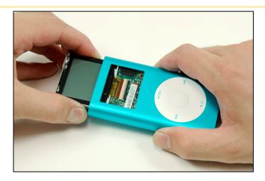
After pushing the logic board out sufficiently, gently grasp the logic board on either side of the display, and continue to slide the iPod out of its casing.
