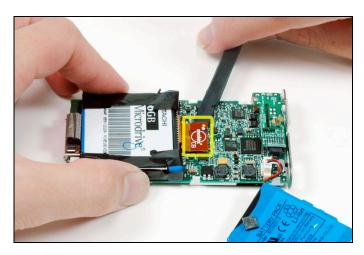
• Use a spudger or the tip of your finger to carefully disconect the orange hard drive ribbon from the logic board.
