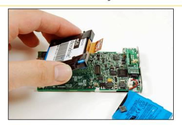
• Lift the hard drive out of the iPod.
